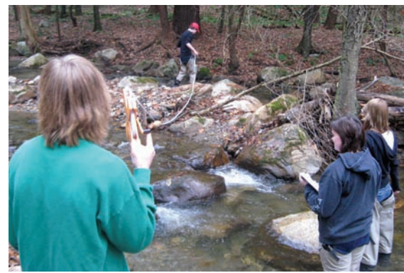
BART students use a tagline to measure the width of Notch Brook
